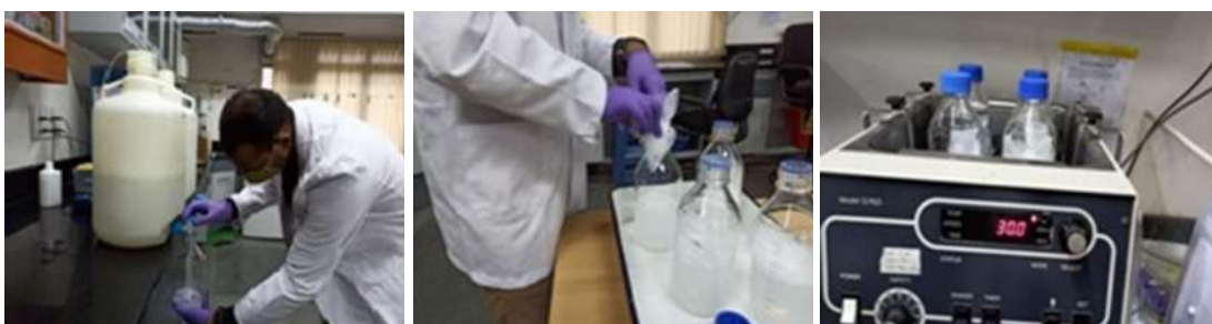
Figure 3.4: Washing of Net samples for regeneration time and wash resistance
