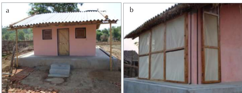
Figure 2.1: Experimental hut (a) Front view showing door and entry windows (b) Rear view showing verandah trap
