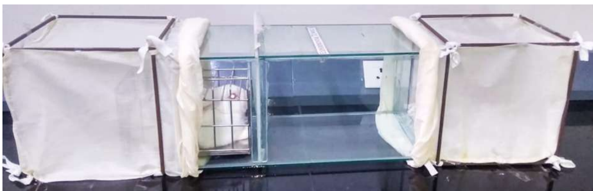
Figure 3.8: A complete set up of a tunnel with mosquito net, cage and rabbit (bait)
