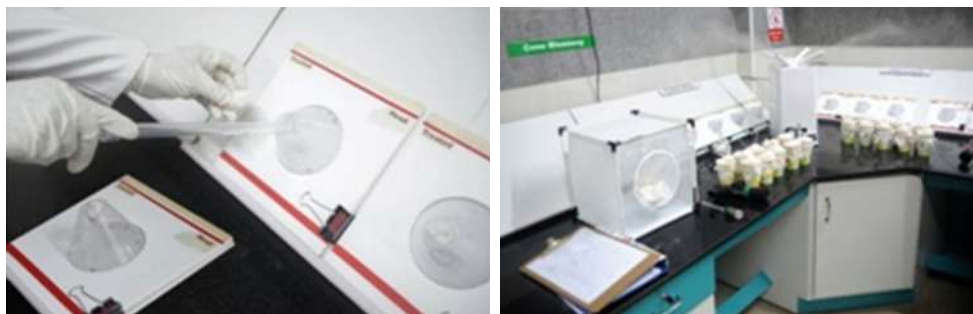
Figure 3.5: Cone bioassay on net samples for regeneration time and wash resistance
